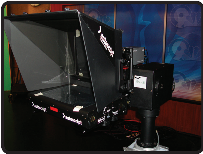
Eagle PT-250 Pan Tilt head shown with Hitachi DK-H32 camera and Autoscript prompter
